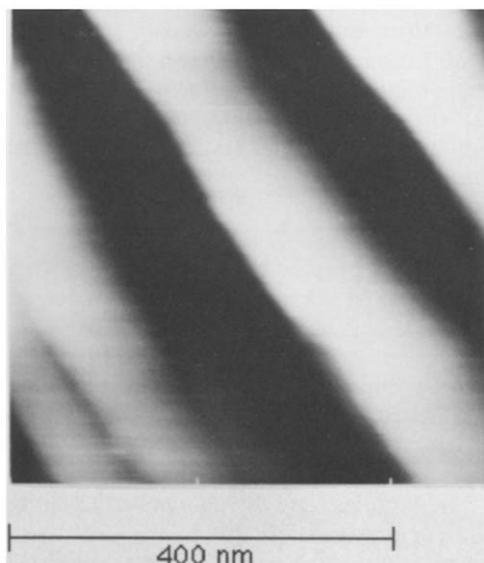
Figure 1 AFM image of microfibrils in oriented polypropylene
